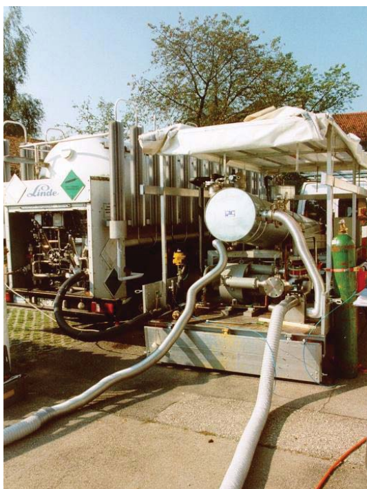
Fig. 4 - Recapture of Vikane using a mobile filter unit.
