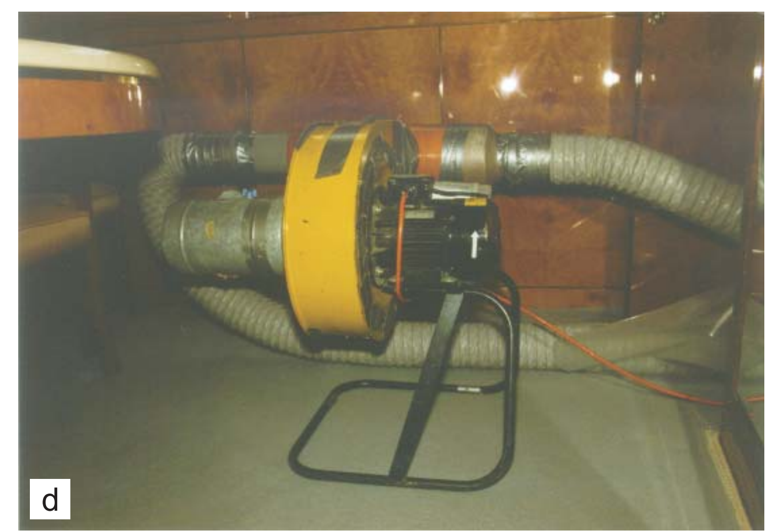
"Tape and seal" technique (a), monitoring the fumigation (b), entering the yacht for aeration (c) and fan with duct-work for gas-distribution (d).
