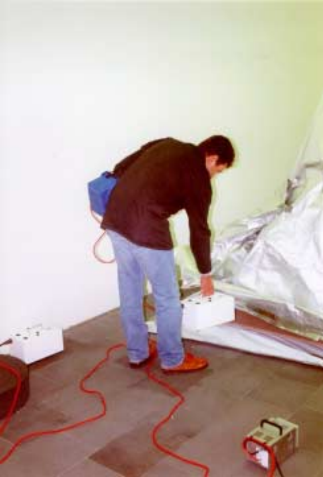
Fig. 8 Detection of Vikane traces for clearance of a fumigation bubble
