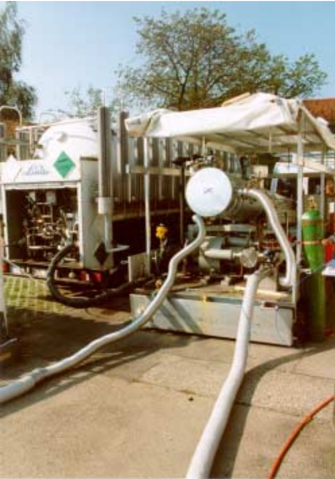
Fig. 7 Recapture of Vikane using a mobile filter unit
